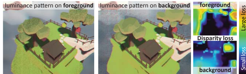
Figure 7.18: To illustrate the prediction of asymmetries, we show two cases: hatching on the foreground ( left ) and the background ( middle ). Compared to foreground hatching (right top), background hatching creates more pronounced differences due to disocclusions, leading to better depth perception (right bottom), as correctly predicted by our metric.
