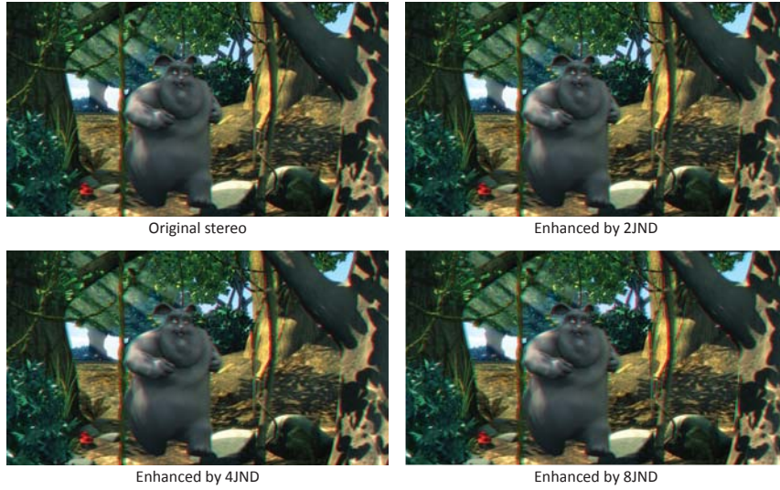
Figure 7.11: We can change the effect of depth perception by increasing JNDs. In this way, we can uniformly exaggerate the depth impression (“Big Buck Bunny” © by Blender Foundation).
