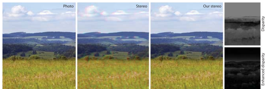
Figure 7.15: Converting a photo (Left) into a 3D image (Middle, anaglyph), just by using the blue channel as depth. Our enhancement (Right, anaglyph) can be used to put stereo cues only where depth contrast exists, minimizing the global error due to the naïve 3D reconstruction, but with locally plausible cues. The insets on the right depict the corresponding disparity maps.
